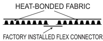
Fig 2. Heat-Bonded
