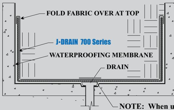
**NOTE:** When using J•DRAIN 700 series cut and remove drainage core and cover with an aluminum plate as shown.
