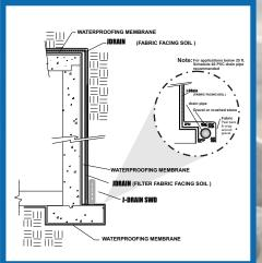
J-DRAIN 150 Core Only consists of a impermeable polymeric sheet cuspated under heat and pressure to form a high flow, high compressive strength dimpled drainage core. J-DRAIN 150 Core Only conveys groundwater seepage from the tunnel wall and away from concrete for the tunnel lining.
